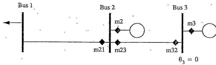
$$x_{12} = 0.1 \text{ pu} \quad \& \quad x_{23} = 0.2 \text{ pu}$$
